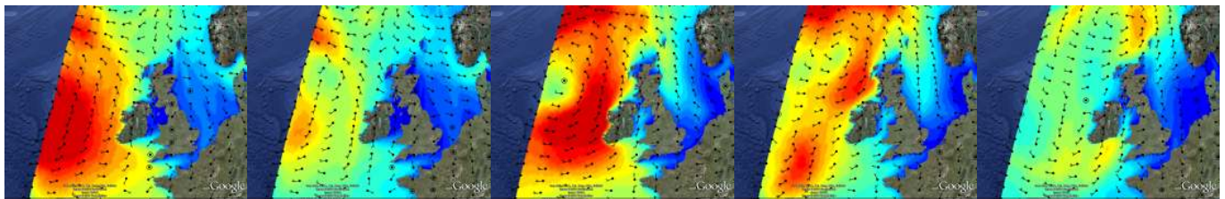
Example: The time series plot from an offshore location in the west shows falling mean sea level (MSL) atmospheric pressure in the coming days; the blues and reds of the plot indicate the trend of the forecast in comparison to previous forecasts, as it is updated. The filmstrip shows the changing wind field and the resulting patterns of increasing wave height as the system passes, later returning to calmer conditions.
